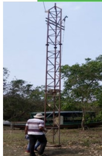
Eddy-covariance flux tower at Bhitarkanika for real-time CO 2 , CH 4 assessment
